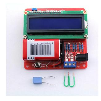
The test 4 (T4) will finish only automatically if you separate the test ports (release connection). You should not touch to any of the test ports or connected cables when calibration is done.
